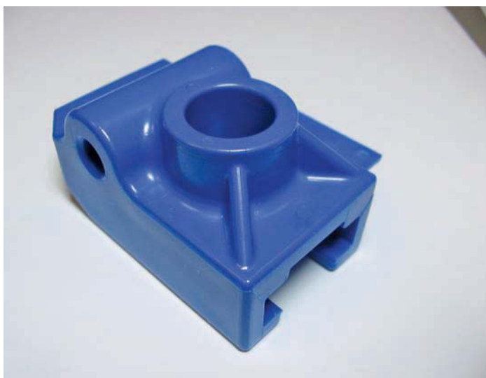
FIGURE 3.19 (a) The 3-D CAD wireframe part model. (b) The injection molded part in the mold. (c) The resulting rapid injection molded part. Courtesy Proto Labs, Inc.
