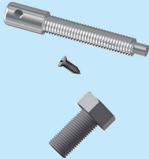
FIGURE 11.41 Examples of solid part models with threads created using a COIL, HELIX, or similar tool.
