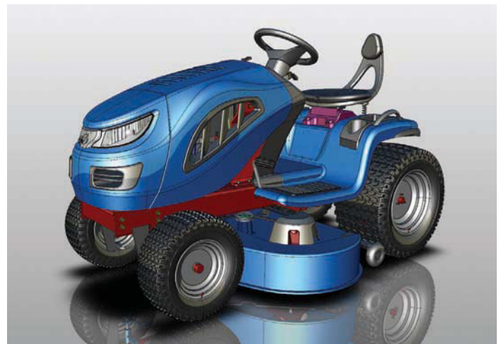
FIGURE 3.51 A lawnmower assembly model that references multiple part and subassembly models. Courtesy Kubotek USA
