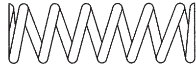
FIGURE 11.93 Step 3: Connect the coils to complete the detailed spring representation.
