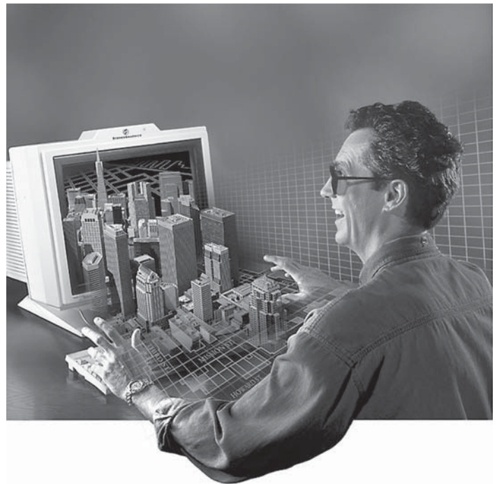
FIGURE 3.30 This lightweight eyewear, a special monitor, and sensing devices generate alternating images, allowing you to see in 3-D. Courtesy StereoGraphics Corporation
