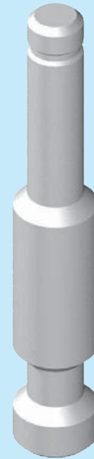
FIGURE 4.80 An example of a revolved feature that will be manufactured using a lathe. This part was modeled using a revolved feature tool. Revolutions are ideal for simulating the use of a lathe to manufacture a product.
