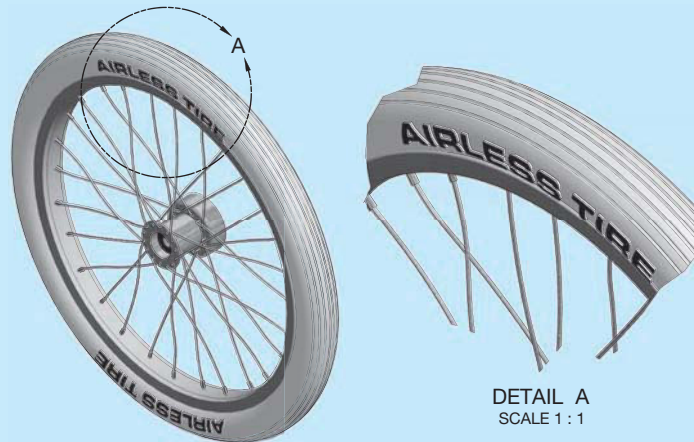
FIGURE 6.44 Text applied to a solid model as an embossment. Notice how the text forms along a circle, which is easy to accomplish using CADD.
