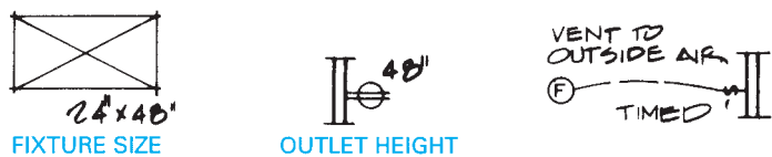
FIGURE 20.26 Special notes for electrical fixtures. © Cengage Learning 2012
