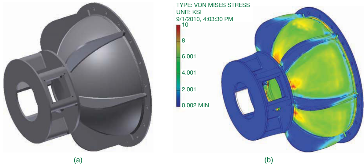
FIGURE 3.63 (a) The design of the initial digital prototype of the endcap. (b) A simulation of the resulting design under the loads from internal pressure.
